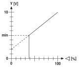
Control with 4...20 mA via external resistor
