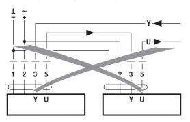
Control with 4...20 mA via external resistor
