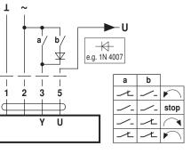
Override control and limiting with AC 24 V with rotary switch
